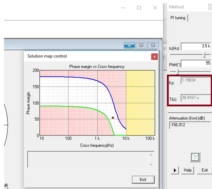
Figure 13: Kp and Ti values extracted from SmartCtrl
