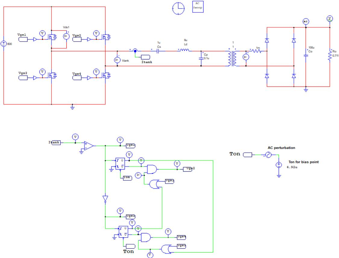
Figure 2: Circuit schematic including the AC sweep
