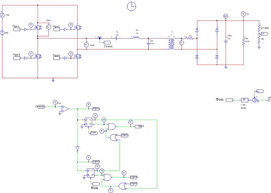
Figure 14: Psim schematic including a input voltage step
