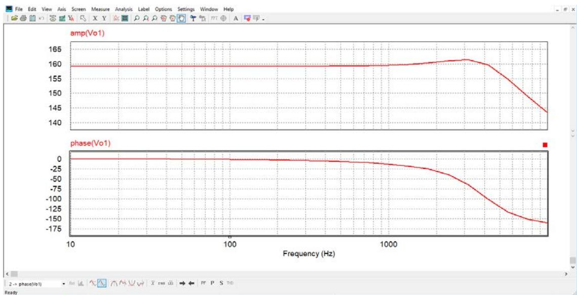
Figure 3: Frequency response of the resonant converter
